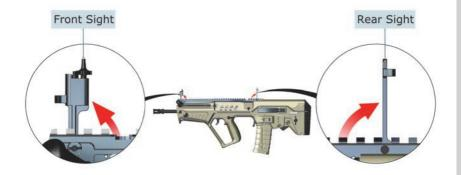
Folding front and rear backup sights are of blade and aperture type respectively, which enables aiming by viewing the blade through the aperture, and visually centering the top of the blade in the aperture.
