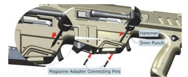
2. Remove the adapter assembly from the rifle body.
