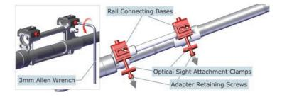
2. Separate the barrel unit from the connecting bases.
