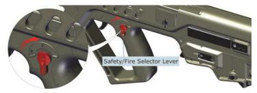
2. On the rifle left-hand side, depress the safety plunger with a 1.5mm punch and slide the fire selector lever off the safety assembly.
