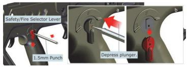
3. On the rifle right-hand side, depress the safety plunger with a 1.5mm punch and slide the safety pivot cover off the safety assembly.
