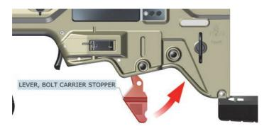
3. Push the locking pins all the way into the body to secure the sear mechanism and the bolt carrier stop lever in place.
