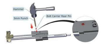
4. Install the general pin on the left side of the bolt carrier using a 3mm punch and a hammer.
