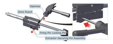
2. Remove the firing pin from the breech block.
