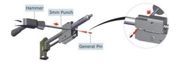
2. Using a 3mm punch and a hammer, remove the rear bolt carrier pin from the right side of the bolt carrier.
