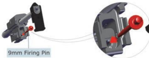
2. Using a hammer and a 3mm punch, push the firing pin locking pin all the way into the breech block.
