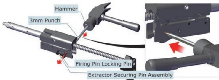
2. Remove the firing pin from the breech block.
