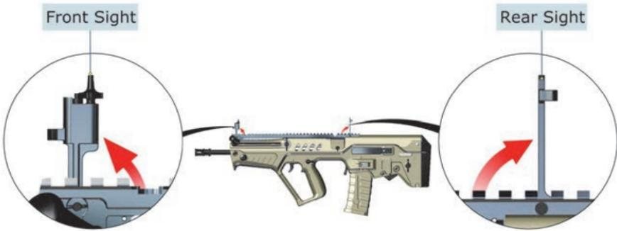
Folding front and rear backup sights are of blade and aperture type respectively, which enables aiming by viewing the blade through the aperture, and visually centering the top of the blade in the aperture.
