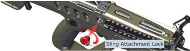
3. Insert the cotter pin into the sling attachment lock.
