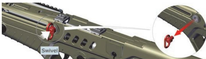
2. Insert a 3mm punch in the eye of the cotter pin and pull the pin out of its recess in the sling attachment lock.
