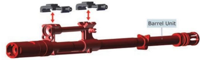
2. Tighten the adapter retaining screws on their bases using a 3mm Allen wrench.
