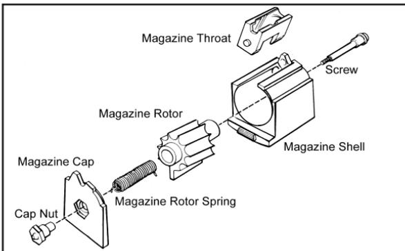
Exploded view of the 10/22 magazine components. This illustration is included to show the relationship and names of the magazine components. As noted in the text above, the magazine should not be disassembled.
