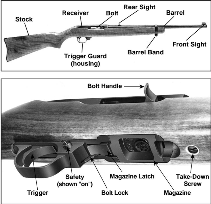
**Figure 1.** In these illustrations the frequently used operating components are identified. Note that the safety is protruding fully from the right side of the trigger guard and is therefore in its “on” (safe) position.
