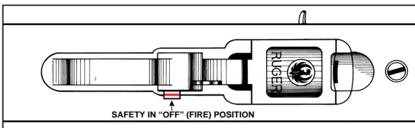
**Figure 2.** The underside of the trigger guard section of the rifle. In this illustration the safety is shown in the “off” (fire) position. The position of the safety and red band indicate the safety is “off.” **It should be in this position only when you are actually firing at a target.**
